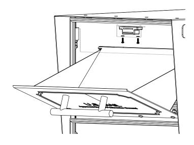
Align the new magnet into position and attach with the provided hardware.
