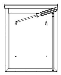
While the mailbox is hanging on the top screws, insert the remaining two screws into the bottom holes and secure with a screwdriver.
