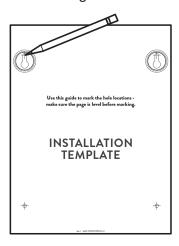
Drill into the wall at each marked location. Use a 1/4" drill bit for brick or other masonry wall. Use a 1/16" drill bit for wood wall.
