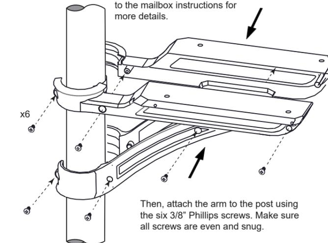
5 TO INSTALL USING TOP MOUNTING HOLES
