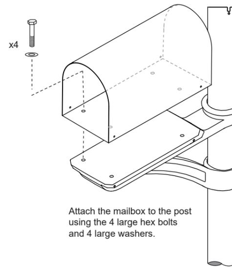
TO INSTALL USING SIDE MOUNTING HOLES
